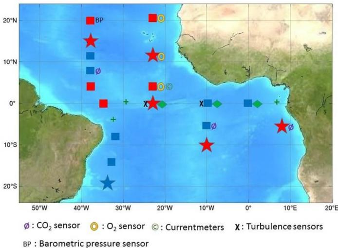
*The present PIRATA network: the meteo-oceanic buoys are represented by rectangles and by stars for Full Flux ones. T-Flex are colored in red and ATLAS in blue. ADCP moorings are represented by green diamonds. Additional symbols are explained in the map legend. All meteo-oceanic buoys are equipped with OTN. Green crosses represent islands where some tide gauges and meteorological stations are/were also maintained.*
