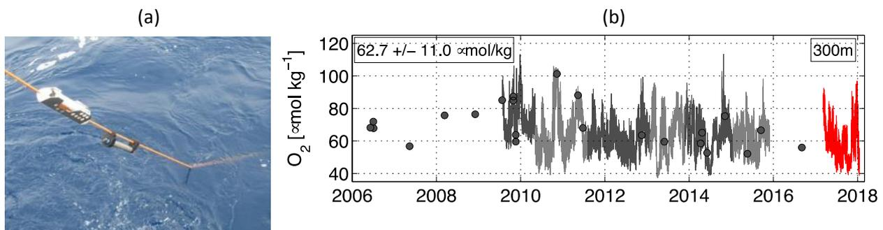
Fig. 2: (a) Deployment of  $O_2$  sensor (instrument closer to water surface) together with MicroCAT during cruise RB-17-01 leg 2. (b) Oxygen time series from the PIRATA mooring site  $11.5^\circ\text{N}$ ,  $23^\circ\text{W}$  at 300 m depth. Dark and light grey lines denote periods of individual mooring periods. Red solid line denotes online  $O_2$  data from the currently deployed PIRATA T-Flex buoy. Dots denote CTD measurements from PIRATA and GEOMAR cruises close to the mooring position.
