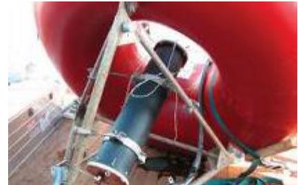
*Fig. 3. a) Old buoy on the left and new T-Flex buoy on the right b) submarine part of the existing CO<sub>2</sub> sensor installed on an old buoy.*
