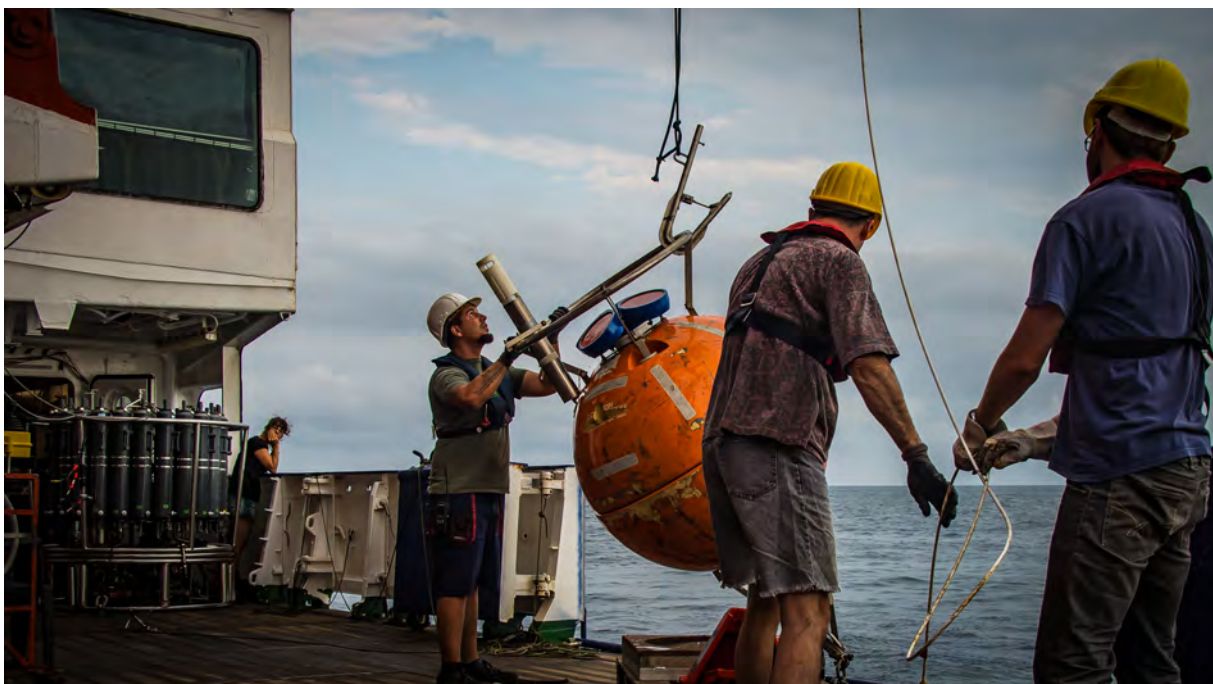
Fig. 2: Recovery of the top element including the acoustic Doppler current profiler of the mooring within the Angola Current at 11°S (photo: SvN).
