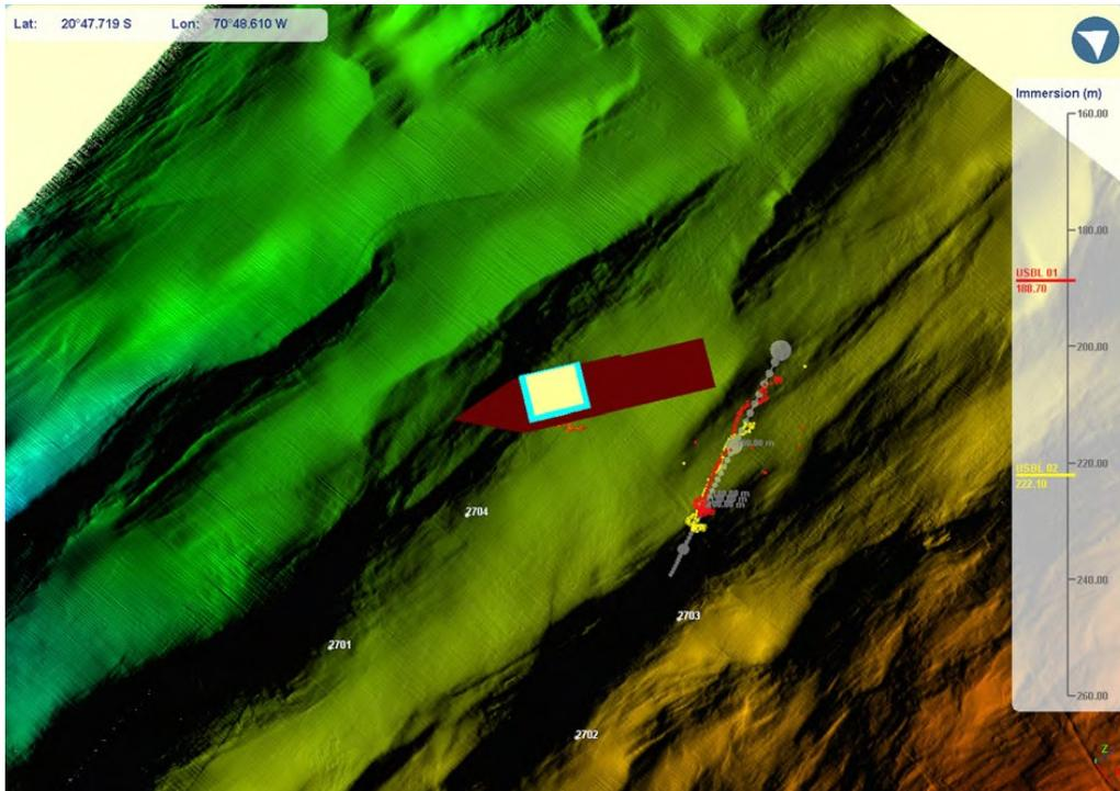
*USBL-Tracker monitoring the distance between two Posidonia transponders (red and yellow) to survey the seafloor deployment – and the yanking off of the tripod. White dots on the seafloor AUV map indicate planned positions of the GeoSEA network.*
