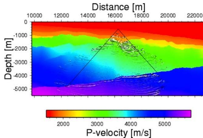
**Figure 3.** Migrated image of target horizons superimposed on the velocity section through the drill site. Seventy receivers at 15.24 m are located between 800 and 2019 m depth for modeling, but a closer spacing and shallower deployment are anticipated in the field. Lines indicate volume imaged inside of diffraction tails.
