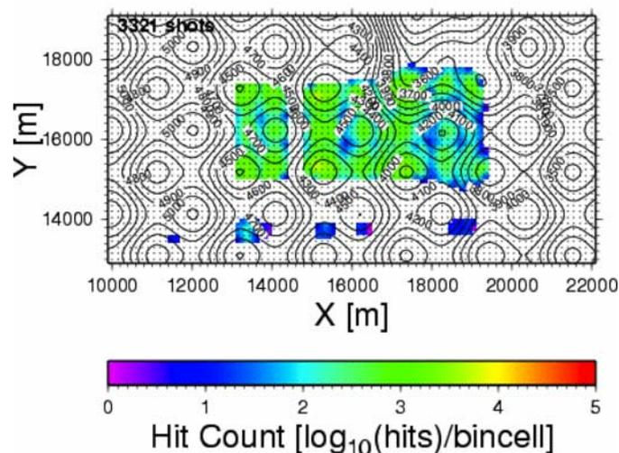
**Figure 6.** Hit map from modeling of a rugose plate interface.
