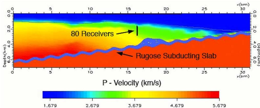
**Figure 5.** Synthetic rugose plate boundary modeled. Larger feature at center represents a 1.5 km high subducted seamount.
