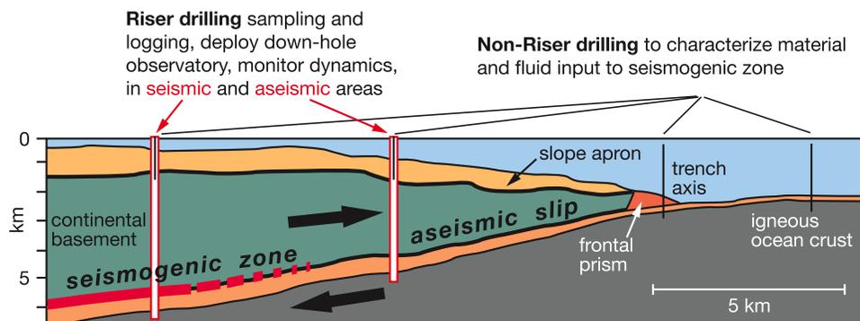
**Figure 2.** The proposed CRISP transect of drill holes showing site 3A in the aseismic zone. Heavy lines indicate target velocity discontinuities entered into the model.
