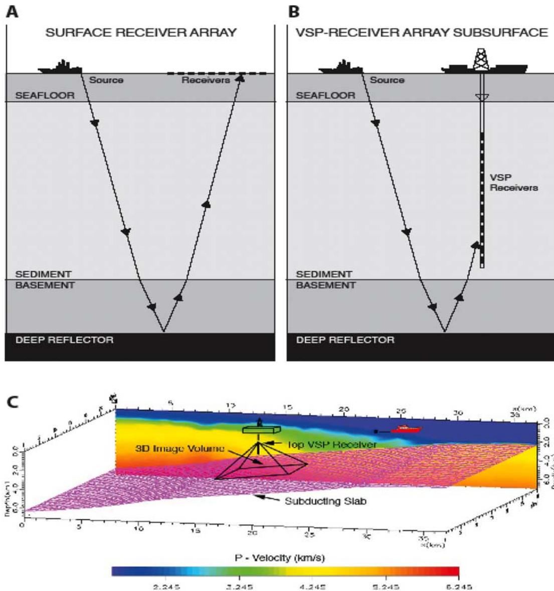
**Figure 1.** (a) Surface receiver acquisition where reflections pass twice through the seafloor and sea surface. (b) VSP array in a borehole below the seafloor. (c) Vertical backdrop is a seismic velocity section from Costa Rica. The pyramid on the subducting slab represents the 3-D volume of seismic data acquired, and its base is the plate interface area imaged. Reflections from a grid of surface signals are received by the vertical geophone array beneath the drill ship.
