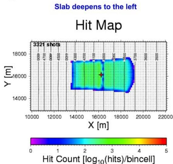
**Figure 4.** Data density shown as a hit map indicating number of seismic source signals received in 100 m bins on the plate boundary or top of the slab. The model assumes a featureless planar plate interface fault at the top of the subduction channel.
