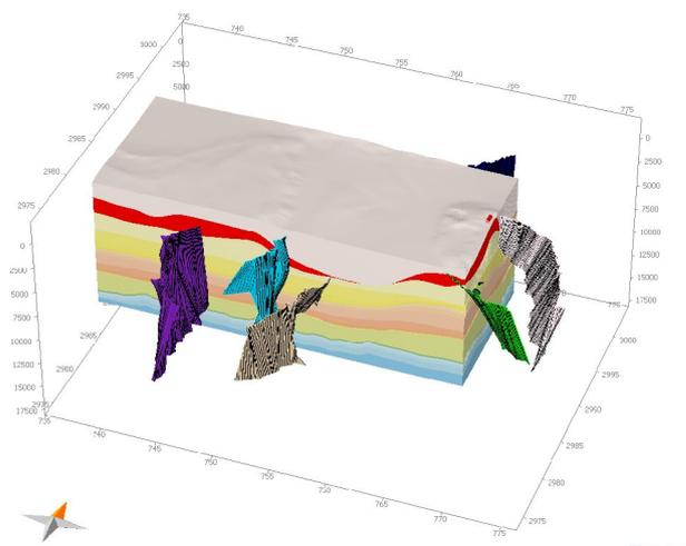
Figure 1: 3D modeling domain, Green Canyon site, Gulf of Mexico. Figure shows sedimentary layers and faulting structures implemented into the model.
