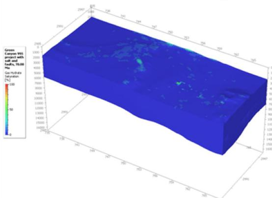
Figure 3: 3D modeling results presenting paleo-gas hydrate accumulations at the chosen age of 70Ma, 61.4 Ma, and 32.3 Ma, respectively.
