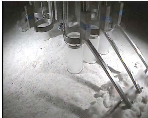
The multi-corer shortly before touching the seafloor and sampling deep sea sediments.
