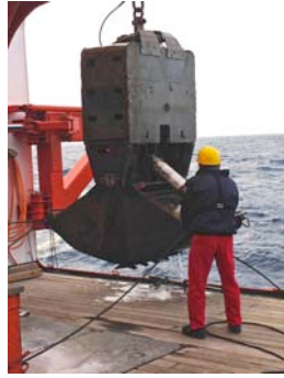
TV grab being deployed from the Sonne with open shovels and back on board with closed shovels and full payload of sediments. (photos: Kaj Hoernle)
