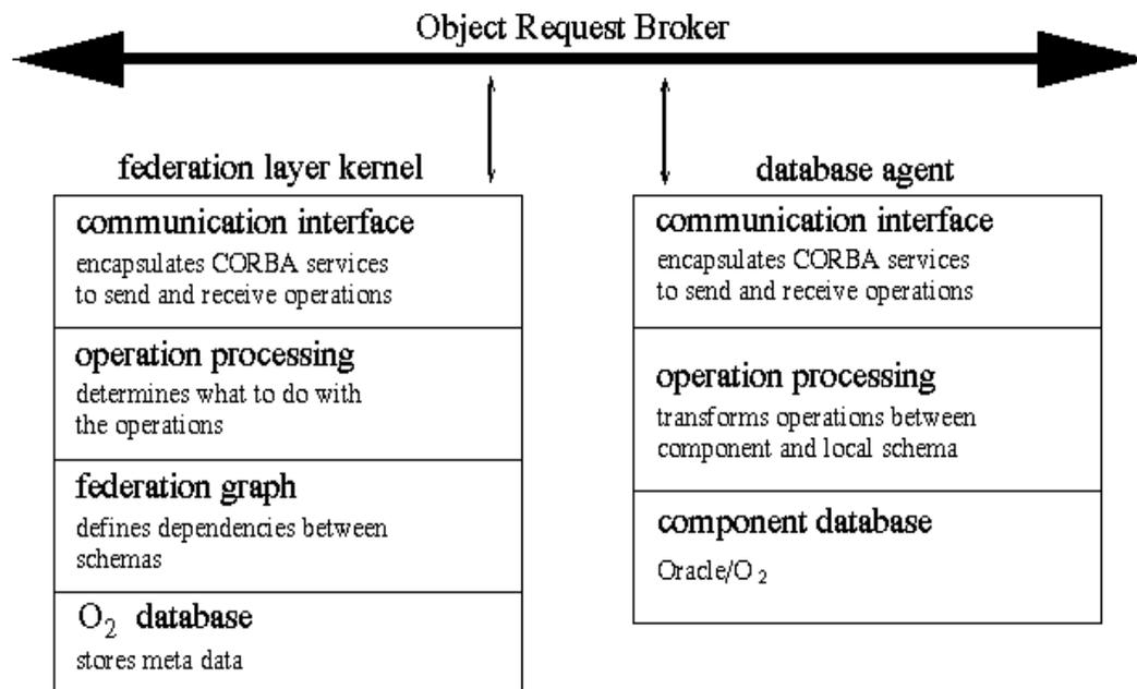
Figure 2: The layers in the CORBA-based architecture of our prototype implementation.
