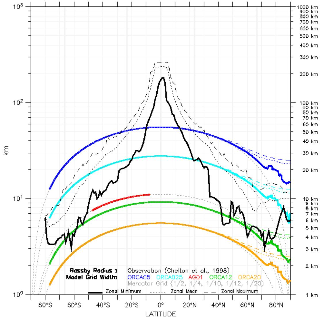
**Figure 1: Internal Rossby radius of deformation proposed by Chelton (1998)(thick black curve), and horizontal grid resolution in various model configuration performed by the IFM-GEOMAR modeling group (figure provided by M. Scheintert).**
