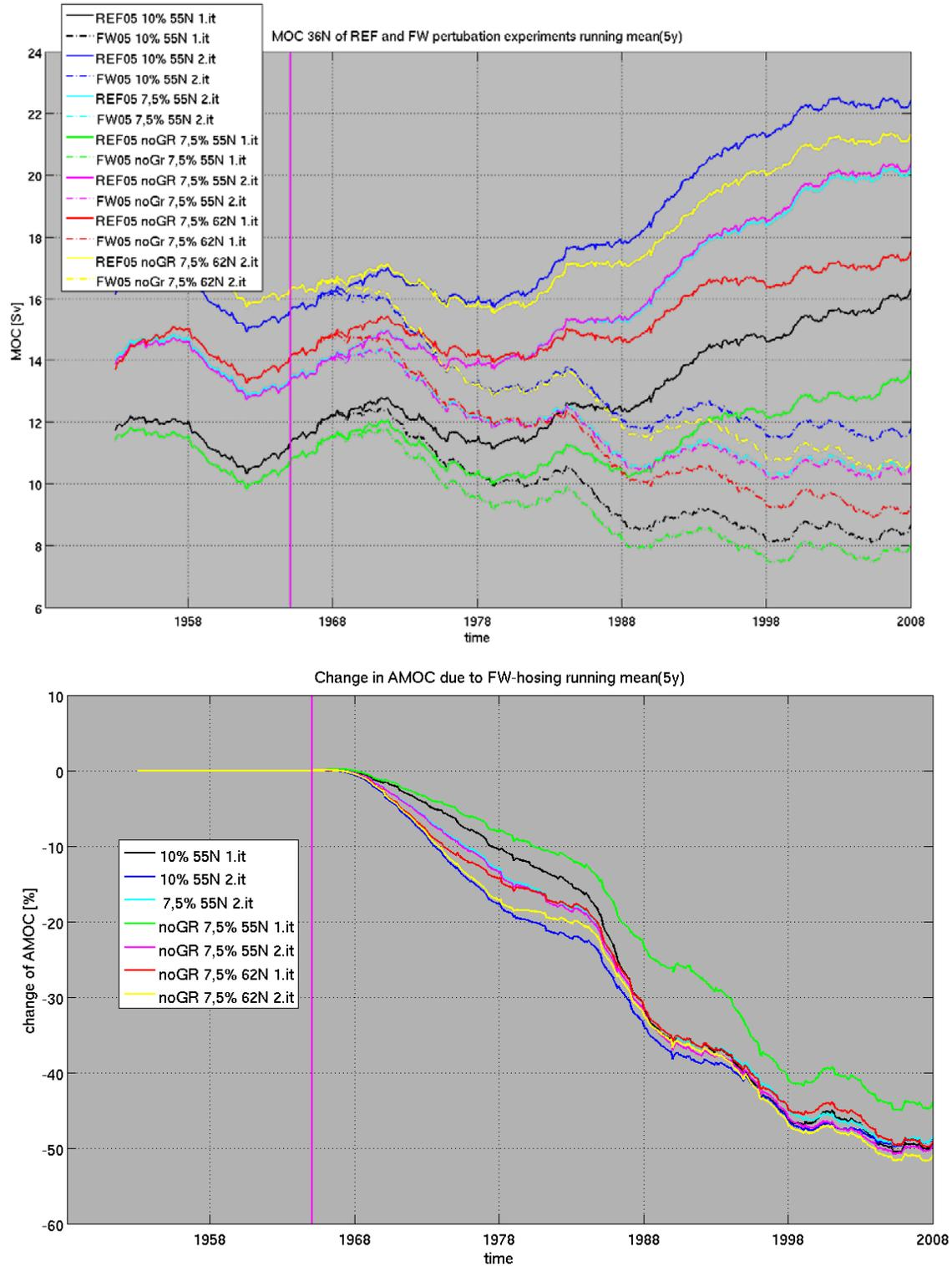
**Figure 4: Impact of the initial state on the reaction to a Melting of Greenland. a) AMOC (36°N) timeseries of reference run (solid) differing in initial states (due to different surface boundary conditions and or different iterations) and corresponding hosing experiments (dashed); b) percentage change of AMOC reaction compared to reference run.**
