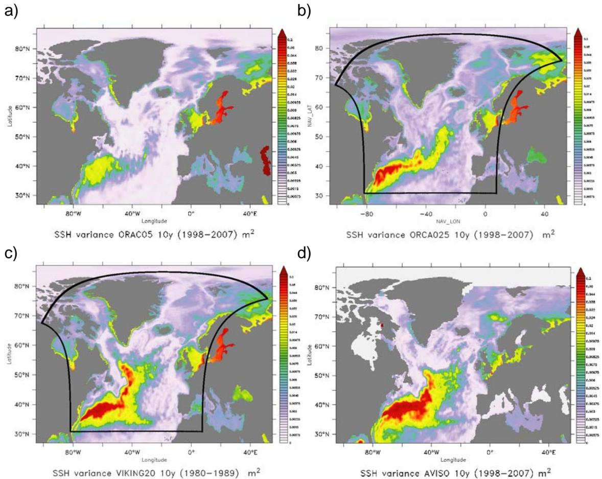
**Figure 2: SSH variability computed over 10 years from 5- daily data for 3 model configurations and observations, ORCA05 (a, coarse), ORCA025 (b, eddy-permitting, box indicate location of high resolution in VIKING20), VIKING20 (c, eddy-resolving, box indicate location of high resolution), AVISO (d)**
